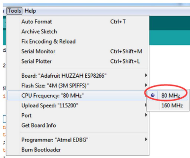
You can keep the **Flash Size** at "4M (3M SPIFFS)". For **Upload Speed**, select 115200 baud .
