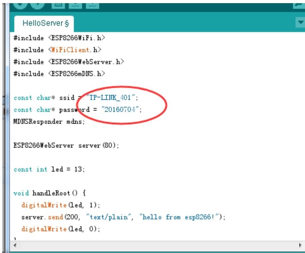
to your access point and password, then upload the same way: get into bootload mode, then upload code via IDE
